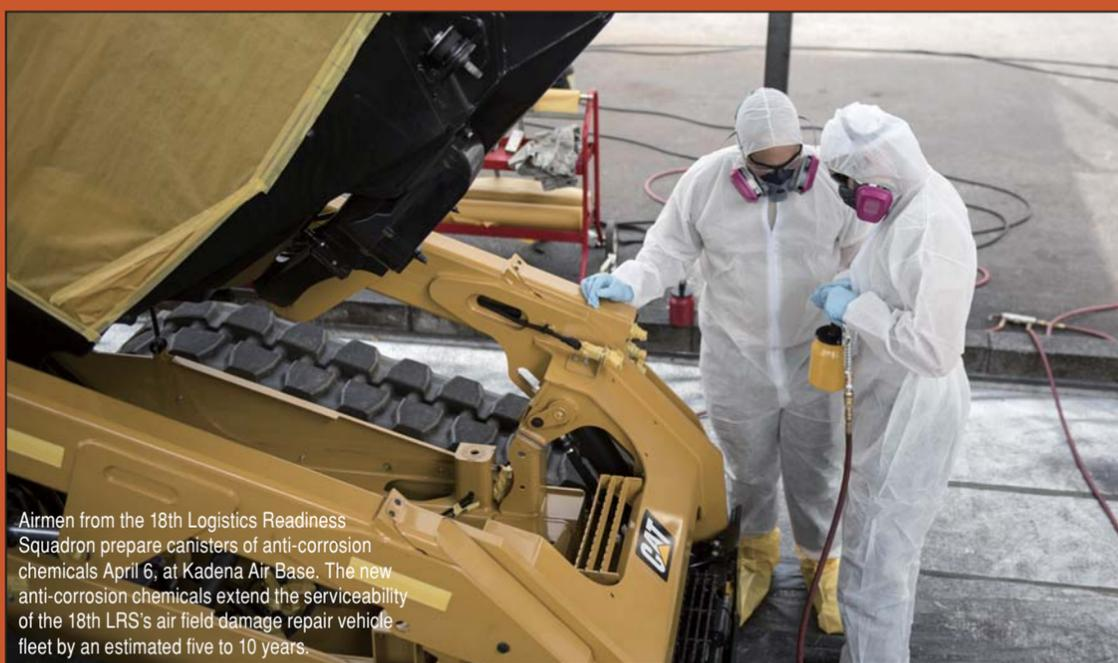
Airmen from the 18th Logistics Readiness Squadron prepare canisters of anti-corrosion chemicals April 6, at Kadena Air Base. The new anti-corrosion chemicals extend the serviceability of the 18th LRS's air field damage repair vehicle fleet by an estimated five to 10 years.
